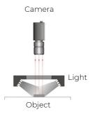
Direct illumination for small objects or where installation space is limited.
