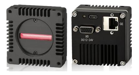
Line scan cameras are a type of camera that captures images one line at a time, unlike regular cameras that capture entire frames at once. They work by using a linear sensor of 1 or 2 pixels high that scans across the field of view. The motion of the sensor or the object being captured creates the second dimension of the image, building up the image one line at a time.
