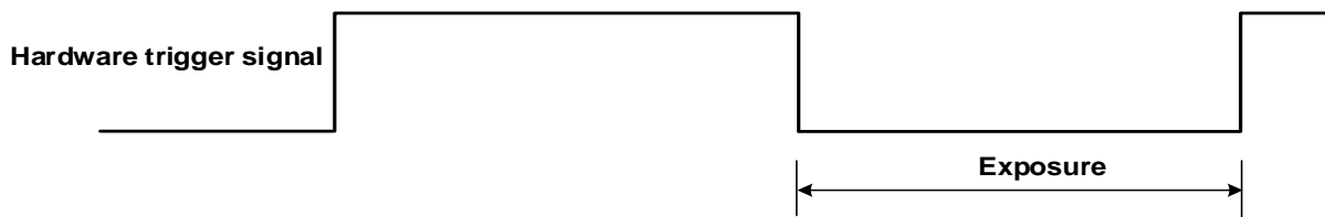
Figure 8-29 The sequence diagram in falling edge trigger of TriggerWidth exposure mode
