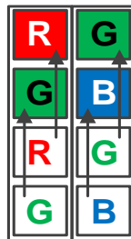
Figure 8-48 Vertical color Binning by 2
