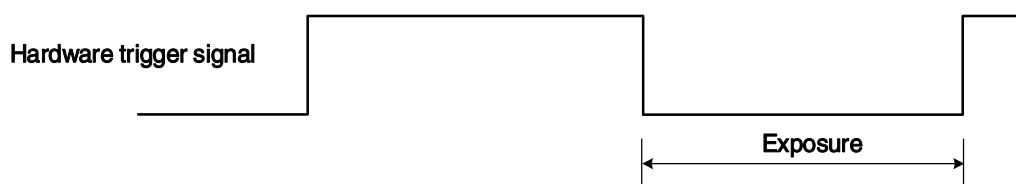
Figure 8-30 The sequence diagram in falling edge trigger of TriggerWidth exposure mode
