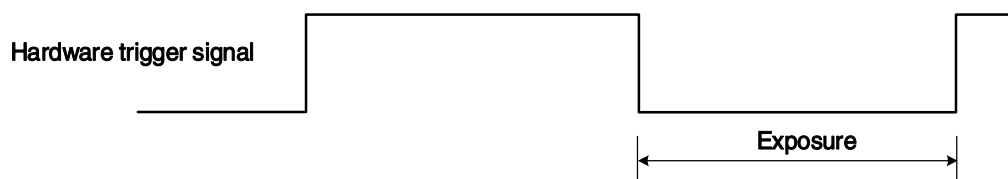
Figure 8-30 The sequence diagram in falling edge trigger of TriggerWidth exposure mode
