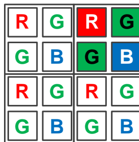
Figure 8-47 Horizontal and vertical color Binning by 2x2
