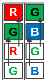
Figure 8-46 Vertical color Binning by 2
