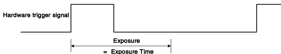
Figure 8-26 The sequence diagram in rising edge trigger of Timed exposure mode
