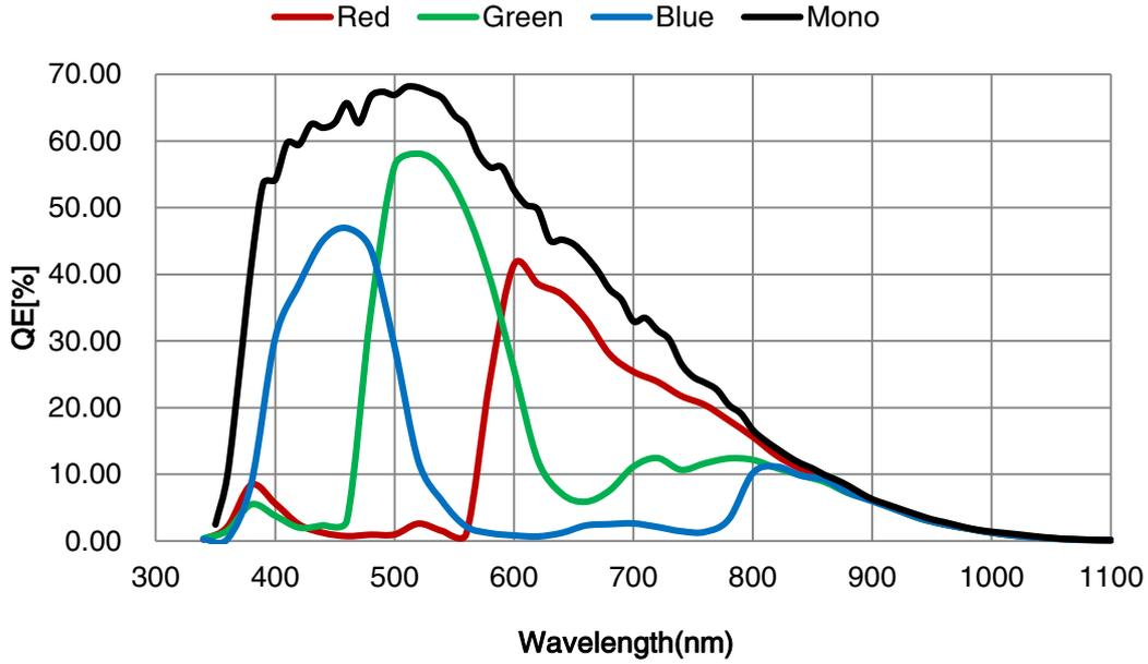
Figure 4-3 MARS-15200-16X2M/C-TF sensor spectral response
