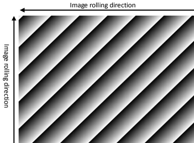
Figure 8-42 Moving diagonal gray gradient test image
