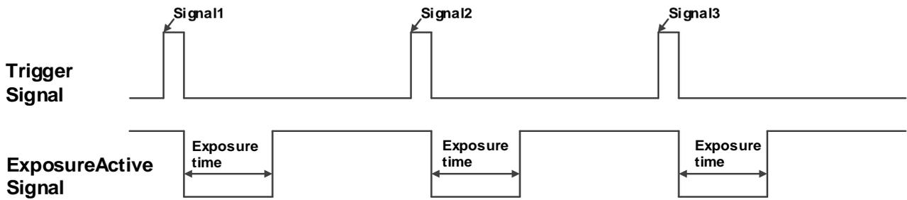
Figure 8-5 Global shutter mode "ExposureActive" signal schematic diagram
