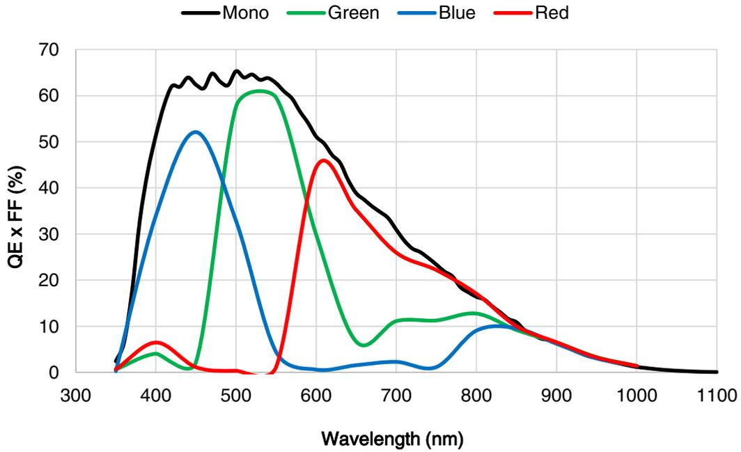
Figure 4-11 MARS-6502-71X2M/C(-NF) \ MARS-6503-71X2M/C(-NF) sensor spectral response
