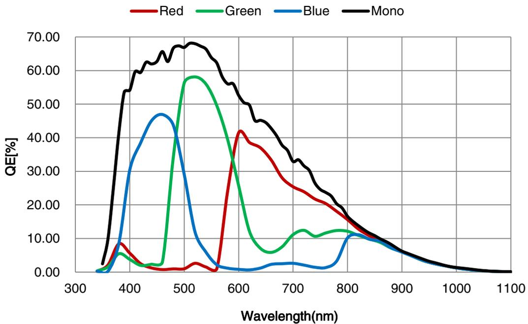
Figure 4-2 MARS-10300-24X2M/C-TF sensor spectral response
