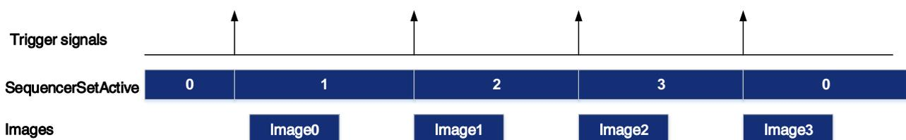
Figure 8-89 Timing diagram
