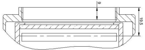
Figure 5-10 Optical interface B
