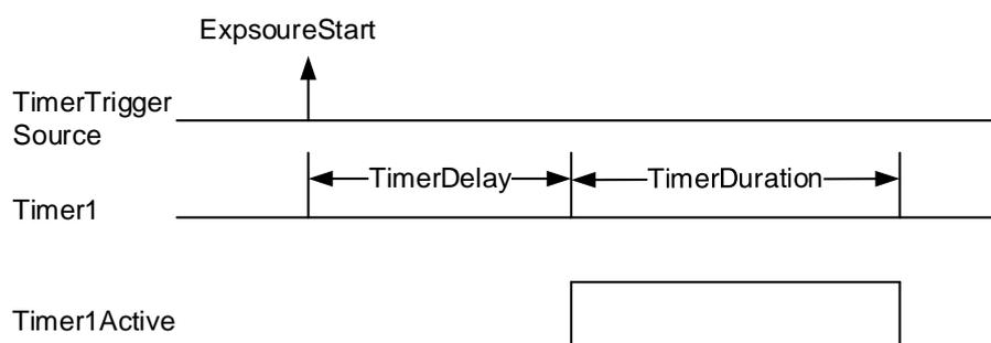
Figure 8-63 Timer1Active schematic diagram
