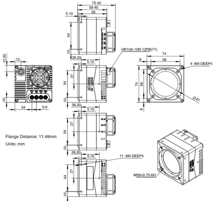
Figure 5-4 MARS-CXP mechanical dimensions D
