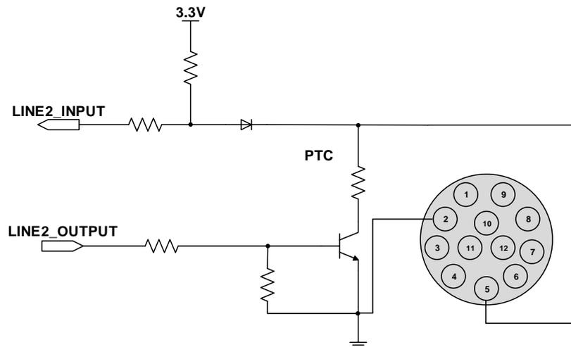
Figure 7-8 GPIO 2/3 (bidirectional) circuit
