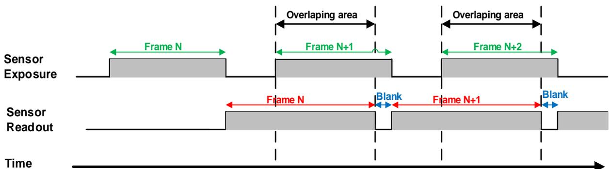
Figure 8-22 The exposure sequence diagram in overlapping exposure mode
