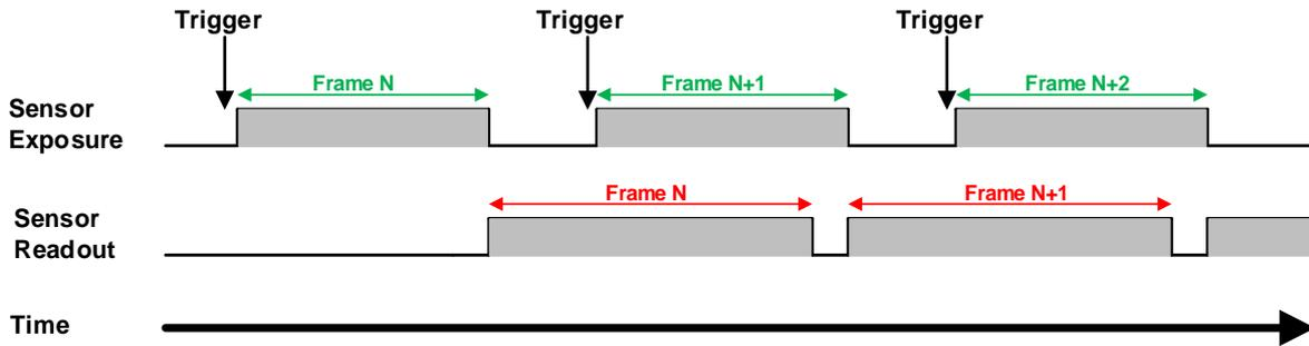
Figure 8-23 The trigger acquisition exposure sequence diagram in overlapping exposure mode
