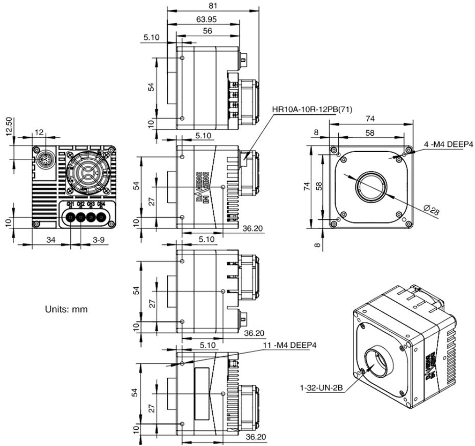
Figure 5-6 MARS-CXP mechanical dimensions F
