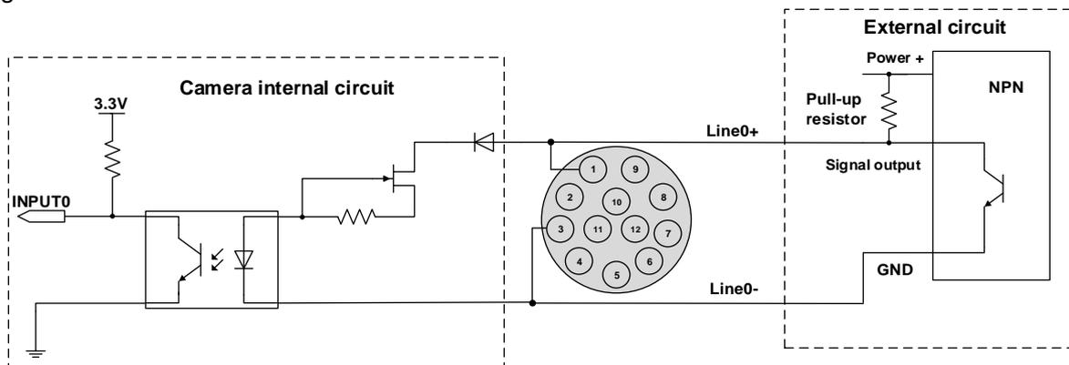
Figure 7-3 NPN photosensor connected to opto-isolated input circuit
