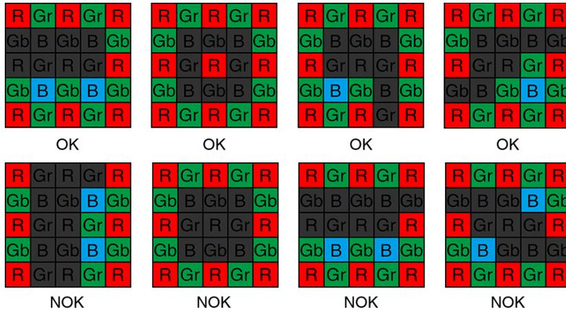
Figure 4-6 MARS-2626-150X2C(-NF) clusters within different Bayer color plane distribution diagram
