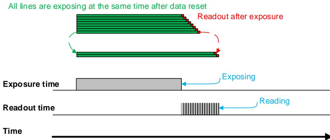
Figure 8-30 Global Reset Release shutter
