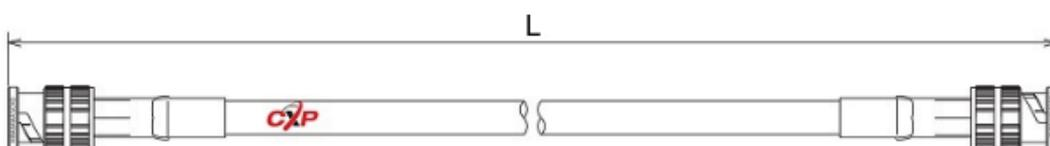
Figure 7-1 the HD-BNC to HD-BNC interface CoaXPress cable
