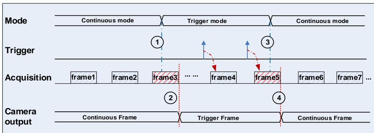
Figure 8-18 Switch trigger mode during frame reading out
