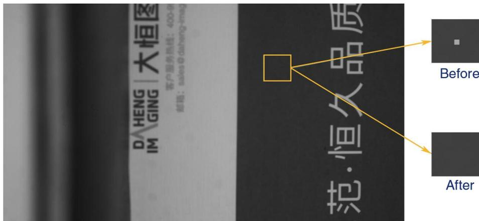
Figure 8-74 Defect pixel correction effect in actual scenario
