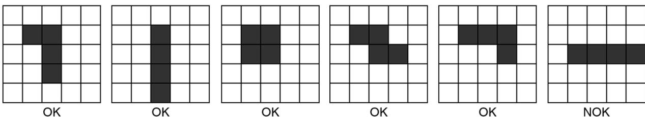
Figure 4-4 MARS-2626-150X2M(-NF) clusters distribution diagram
