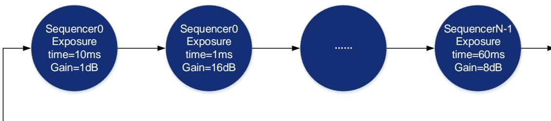
Figure 8-87 Sequencer feature schematic diagram
