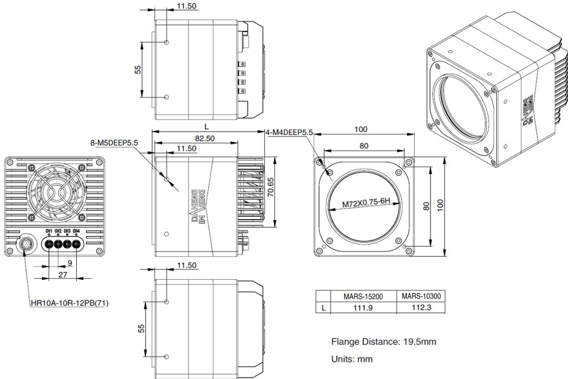
Figure 5-2 MARS-CXP mechanical dimensions B
