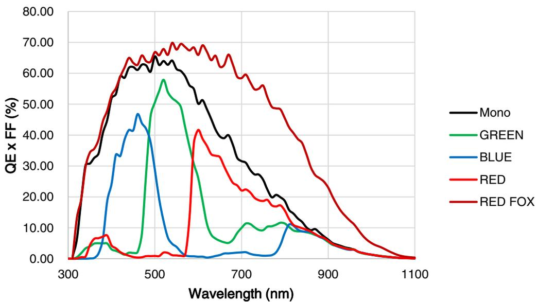
Figure 4-7 MARS-2625-150X2M/C(-NF) \ MARS-2626-150X2M/C(-NF) sensor spectral response
