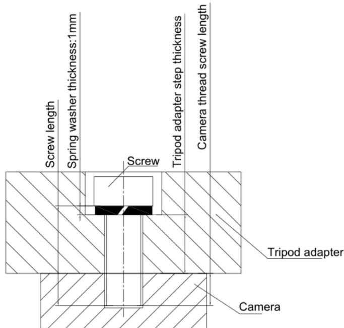
Figure 5-13 Schematic diagram of screw specification, tripod adapter step thickness and spring washer thickness
