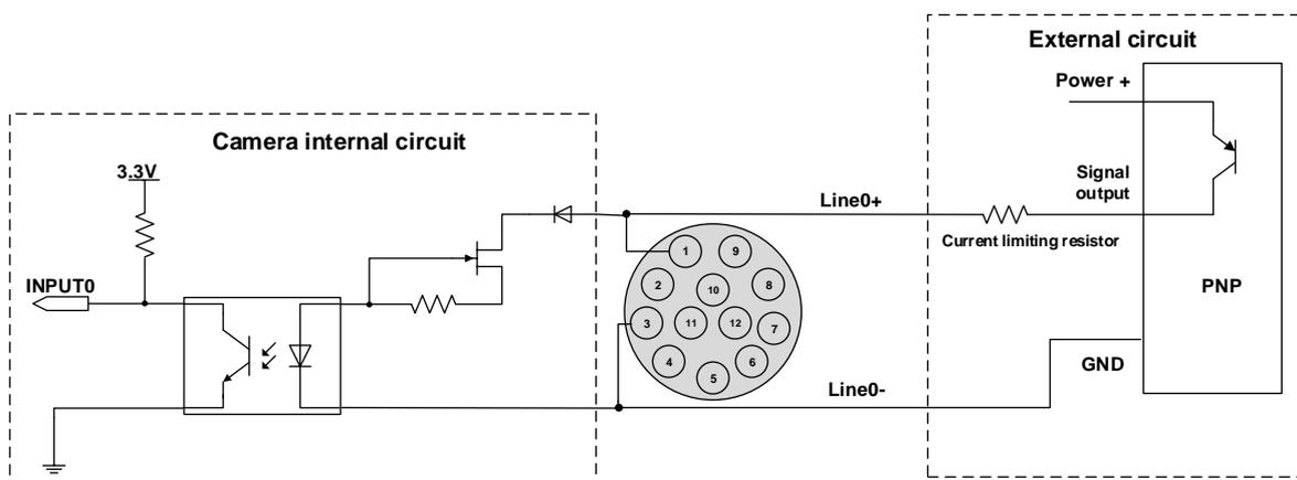
Figure 7-4 PNP photosensor connected to opto-isolated input circuit
