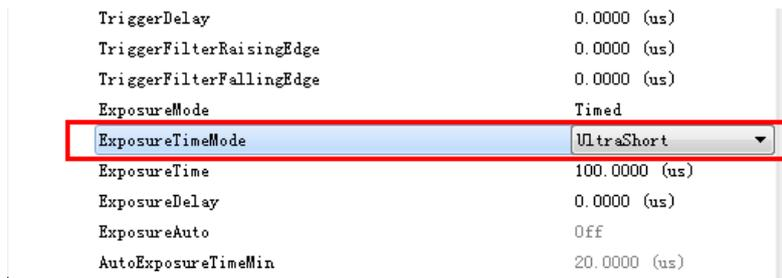
Figure 8-31 UltraShort exposure time mode
