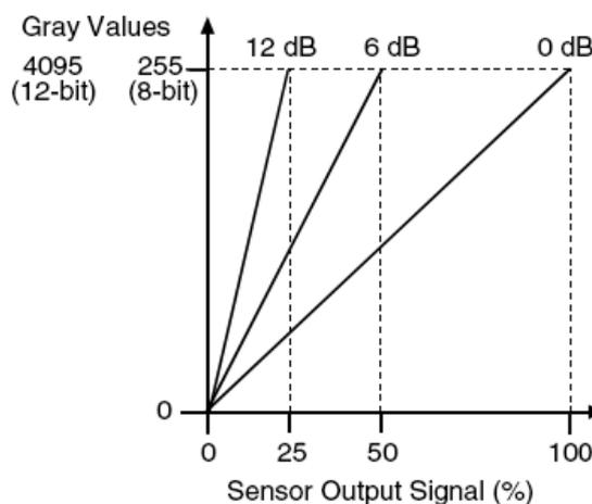
Figure 8-34 The camera's response curve
