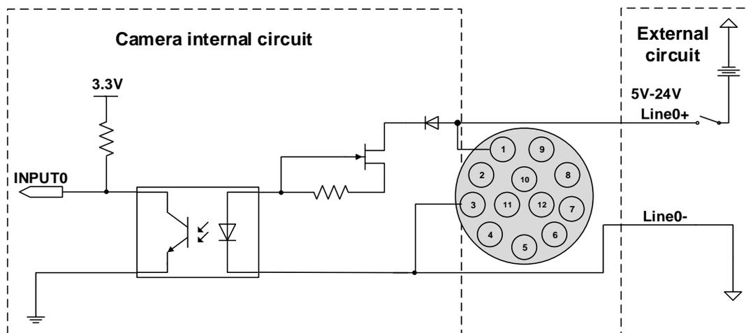
Figure 7-2 Opto-isolated input circuit
