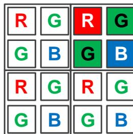
Figure 8-47 Horizontal and vertical color Binning by 2x2
