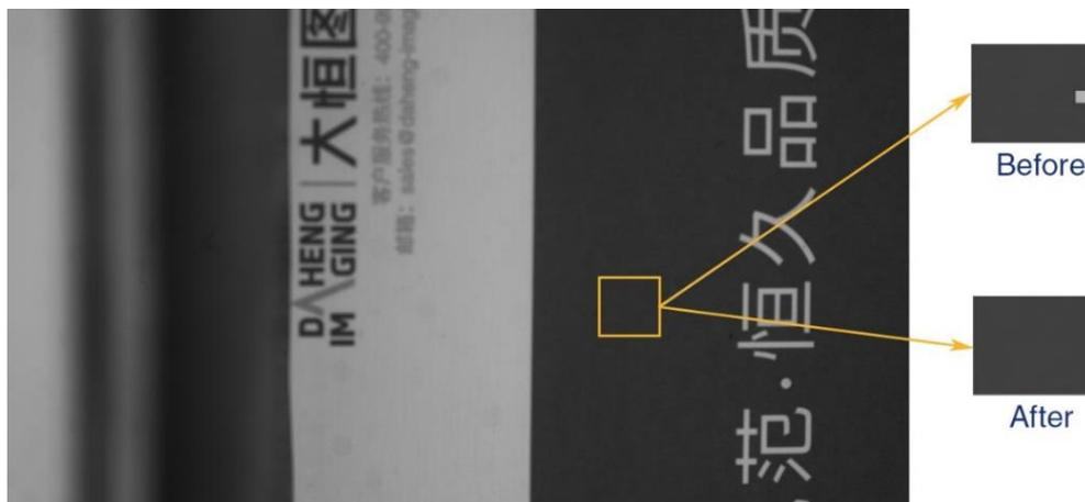
Figure 8-72 Hot pixel correction effect
