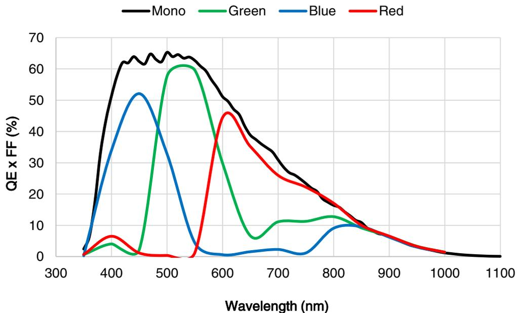
Figure 4-1 MARS-6500-31X2M/C-TF \ MARS-6501-31X2M/C-TF sensor spectral response
