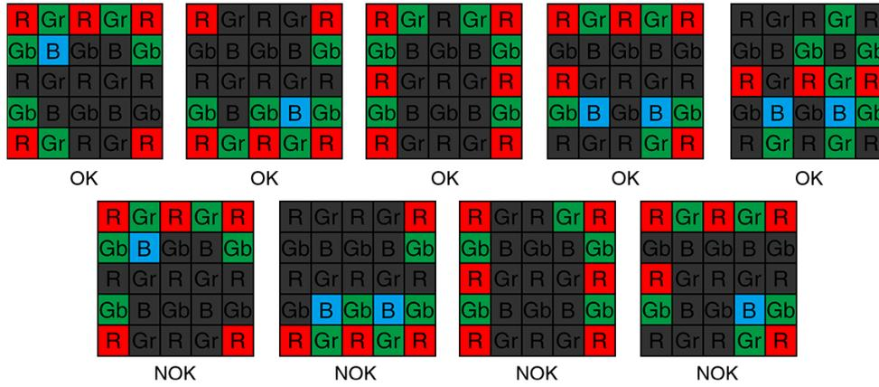
Figure 4-10 MARS-6503-71X2C(-NF) clusters within different Bayer color plane distribution diagram
