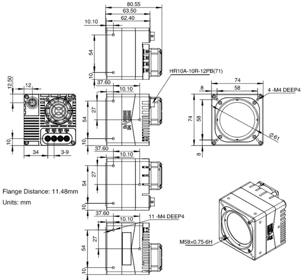
Figure 5-8 MARS-CXP mechanical dimensions H
