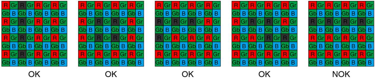
Figure 4-5 MARS-2626-150X2C(-NF) clusters within same Bayer color plane distribution diagram
