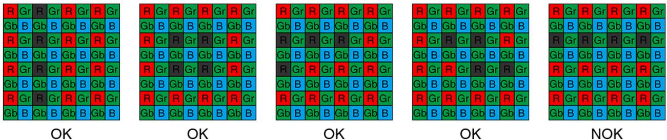
Figure 4-9 MARS-6503-71X2C(-NF) clusters within same Bayer color plane distribution diagram
