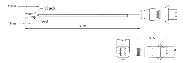
! WARNING! Applying excessive force as well as placing heavy weight on the cable can damage it. Treat the cable carefully and avoid excessive bending, especially when installing it.
