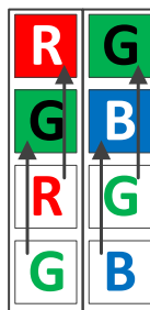
Figure 8-47 Vertical color Binning by 2
