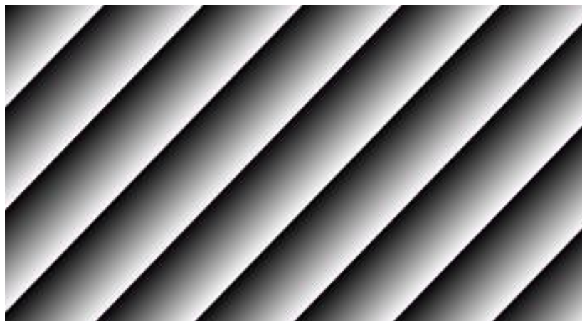
Figure 8-44 Static diagonal gray gradient test image
