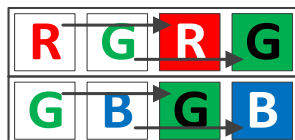
Figure 8-35 Horizontal color Binning by 2
