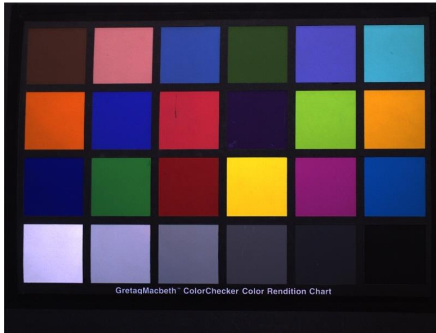
Figure 2-10 Switch on color correction based on figure2-10 (color correction: on; saturation: 64; Gamma: 1; Contrast: 0)
