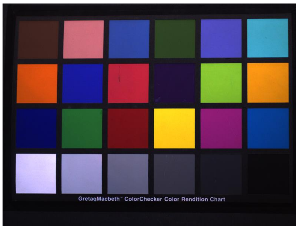
Figure 2-8 Switch on color correction based on figure 2-8 (color correction: on; saturation: 64; Gamma: 1; Contrast: 0)
