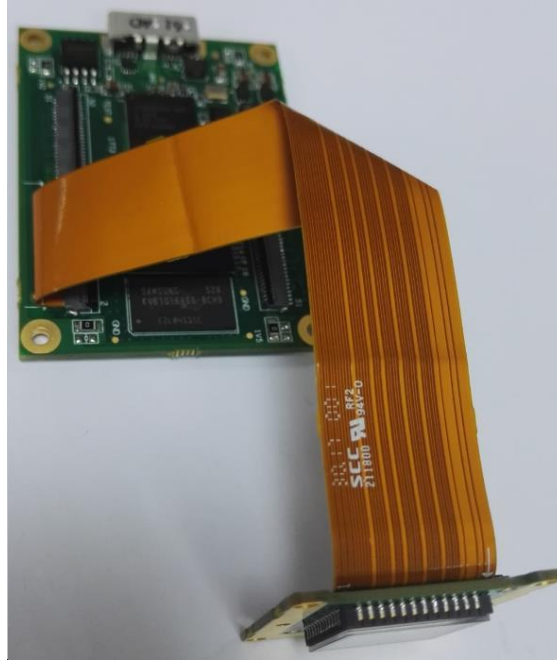
Figure 3-3: Schematic diagram of FPC cable folding and installation
