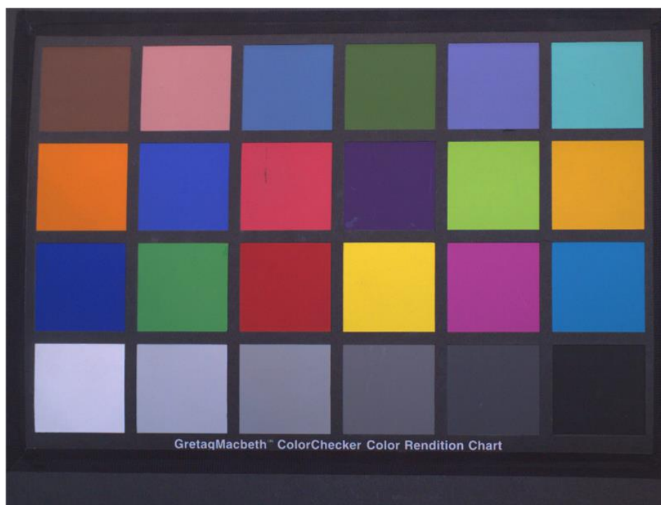
Figure 2-10 Set the Gamma is 1.98(color correction: on; saturation: 80; Gamma: 1.98; Contrast: 0)
