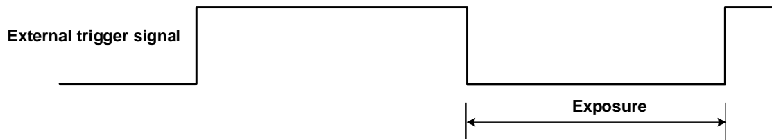
Figure 8-28 The sequence diagram in falling edge trigger of TriggerWidth exposure mode
