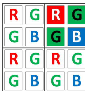
Figure 8-48 Horizontal and vertical color Binning by 2×2
