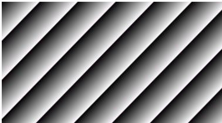
Figure 8-33 Static diagonal gray gradient test image
