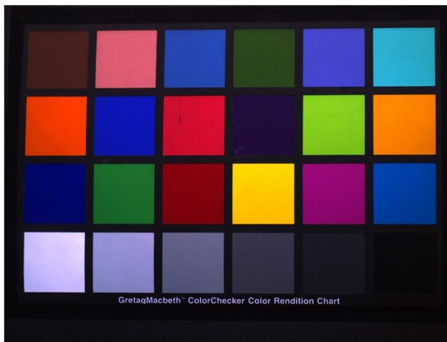
Figure 2-11 Set saturation to 80(color correction: on; saturation: 80; Gamma: 1; Contrast: 0)
