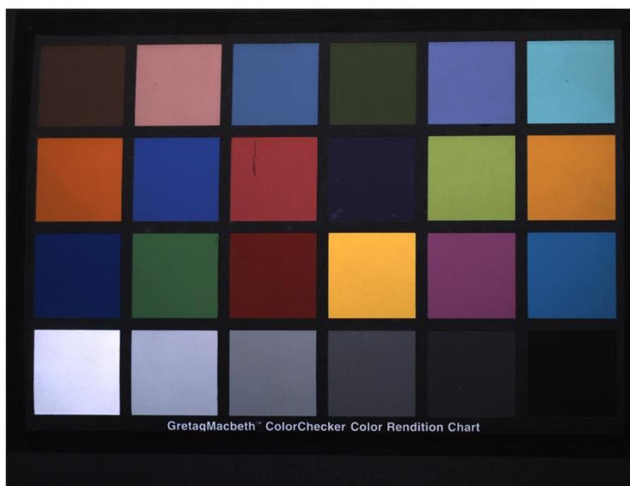
Figure 2-9 Neighborhood interpolation RGB image (color correction: off; saturation: 64; Gamma: 1; contrast: 0)
