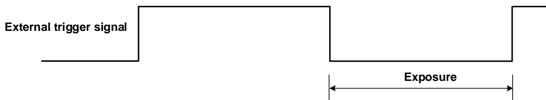
Figure 8-15 The sequence diagram in falling edge trigger of TriggerWidth exposure mode
