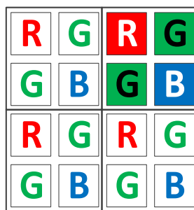
Figure 8-38 Horizontal and vertical color Binning by 2x2
