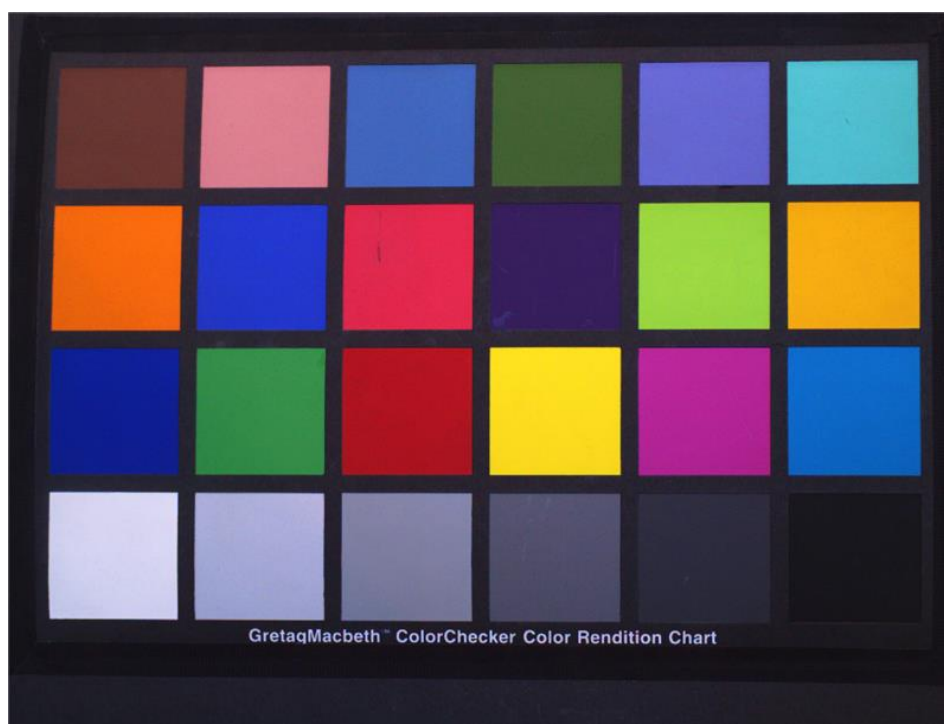
Figure 2-11 Set the contrast is 40(color correction: on; saturation: 80; Gamma: 1.98; Contrast: 40)
